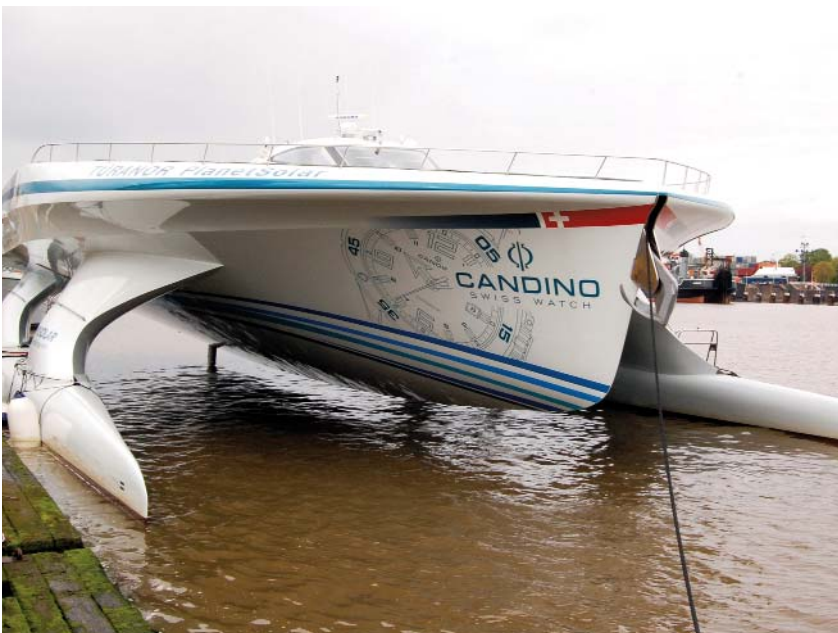
The high-tech Tûranor PlanetSolar, constructed using carbon fibre composites, aims to circumnavigate the world using solar power only. Photo: Reed Exhibitions/Marcus Reichl
